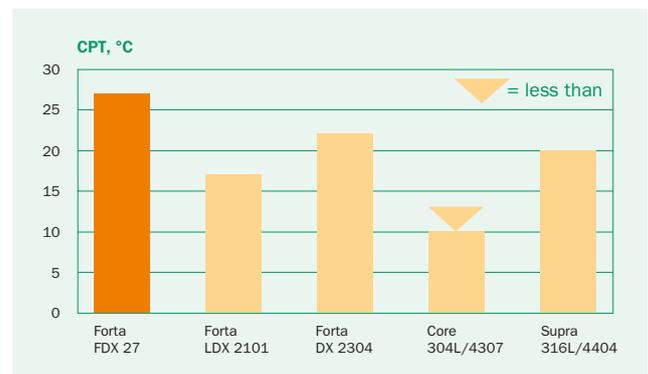
Figure 4. Typical critical pitting corrosion temperatures (CPT) in 1M NaCl measured according to ASTM G150 by using the Avesta Cell. Test surfaces wet ground to P320 mesh. CPT varies with product form and surface finish.
