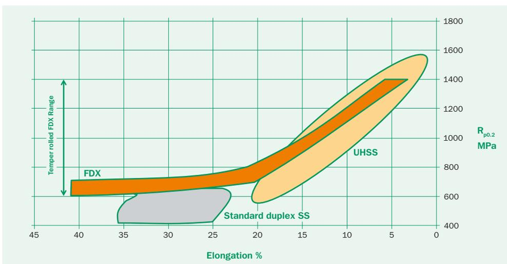
Figure 1. Yield strength and elongation of Forta FDX 27 grades after different levels of cold working compared to standard duplex stainless steels and ultra high strength steels (UHSS).
